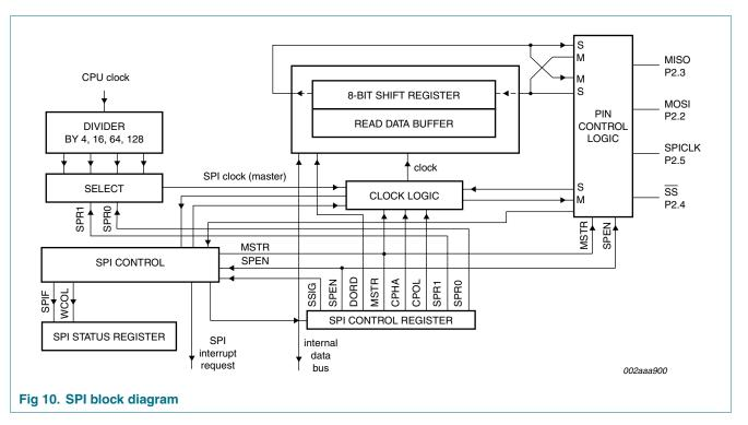
The SPI interface has four pins: SPICLK, MOSI, MISO and  $\overline{SS}$ :
